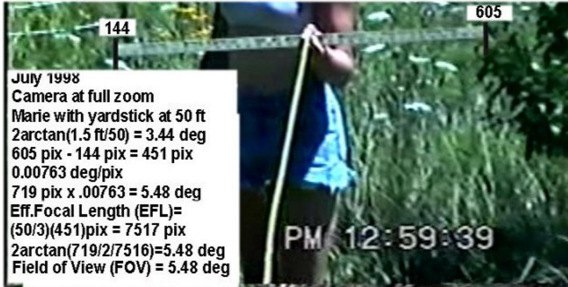
FIGURE 2: CALIBRATION OF THE CAMERA FOR DEGREES PER PIXEL AT FULL ZOOM
