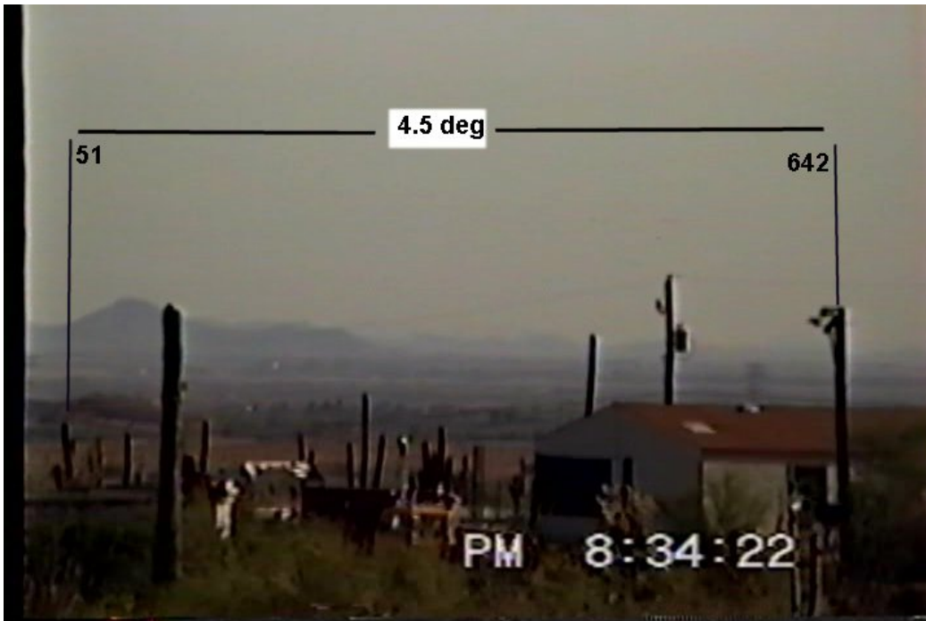
FIGURE 4: SIGHTING DIRECTION TRANSFER FROM "REFERENCE CACTUS" TO "REFERENCE POLE"
